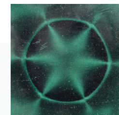
Magnet magnetized at inner periphery
