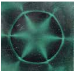
Magnet magnetized at inner periphery
