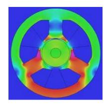
In contrast, bonded magnets with an inherent lower flux density do not saturate the stator's silicon steel. Additionally, the low electrical conductivity of bonded neo magnets minimizes eddy current losses, further reducing vibration and noise in the motor.
