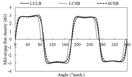
Fig. 5. Simulated mid airgap flux density using closed circuit model
