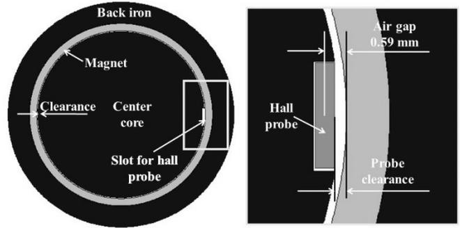
Fig. 4. Closed circuit flux scan set-up
