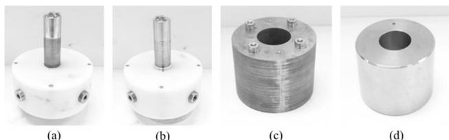
Fig. 6. Fabricated fixture components (a) Laminated fixture core (b) Solid steel fixture core, (c) Laminated back iron and (d) Solid steel back iron
