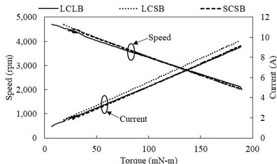
Fig. 11. Motor performance on load
