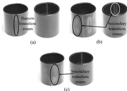
Fig. 10. Magnet pole transition zone (a) LCLB (b) LCSB (c) SCSB
