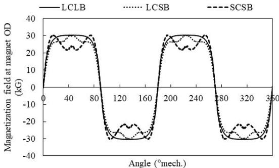
Fig. 3. Applied magnetization field measured at magnet OD
