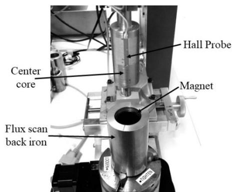
Fig. 7. Closed circuit flux scan measurement set-up
