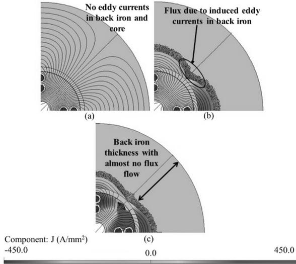
Fig. 2. Flux due to applied magnetization field and induced eddy currents in the fixture (a) LCLB (b) LCSB and (c) SCSB
