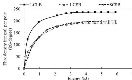
Fig. 9. Magnetization test results for various combinations
