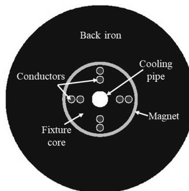
Fig. 1. Magnetization fixture cross-section
