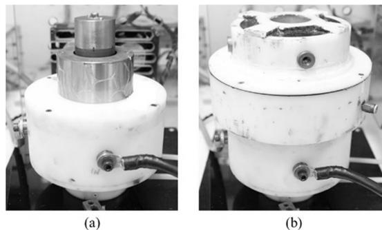
Fig. 7. Fabricated fixtures (a) Inner-only (b) Inner-Outer
