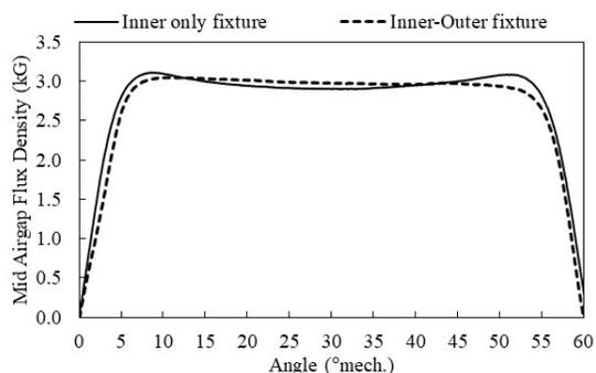
Fig. 10. Measured mid airgap flux density.
