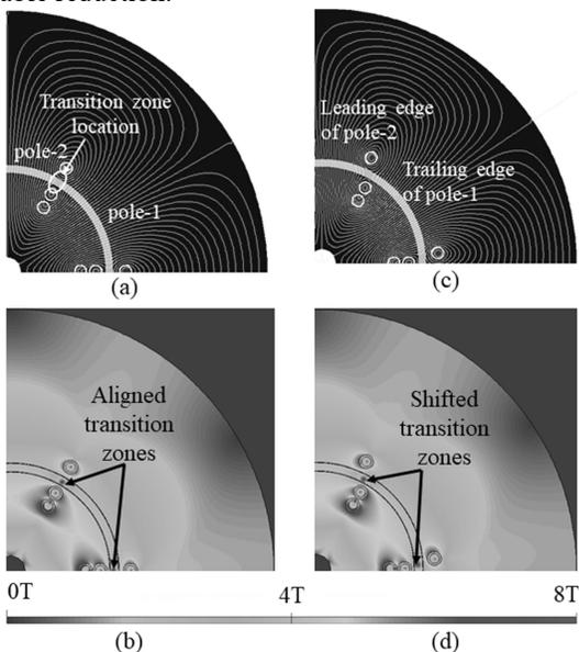
Fig. 5. Inner-outer fixture (a) Magnetization flux, (b) Flux density in aligned position (c) Magnetization flux, (d) Flux density in case of 5° misalignment
