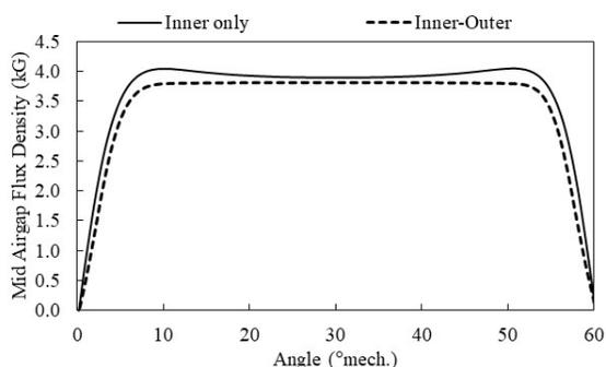
Fig. 3. Mid airgap flux density
