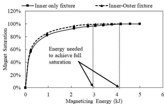
Fig. 9. Saturation test results for inner only and inner-outer magnetization fixtures
