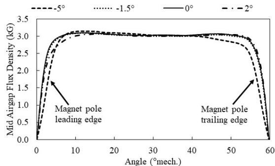
Fig. 11. Measured mid airgap flux for various misalignment positions for a single pole
