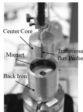
Fig. 8. Closed circuit flux scan measurement set-up
