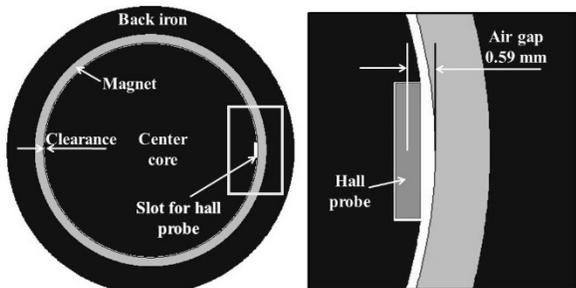
Fig. 2. Closed circuit flux scan set-up
