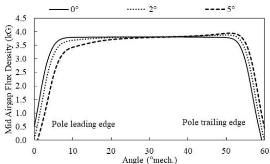
Fig. 6. Simulated mid airgap flux profile for various misalignment angles
