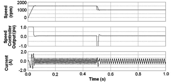
Fig. 2. Reference and actual speed, speed controller output, and line current of the vector-controlled PMSM drive with HPI speed controller based on saturation switching function.
