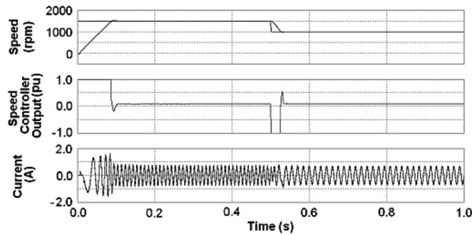
Fig. 5. Reference and actual speed, speed controller output and line current of the vector-controlled PMSM drive with HPI speed controller with switching function based on the output of FEP controller only.
