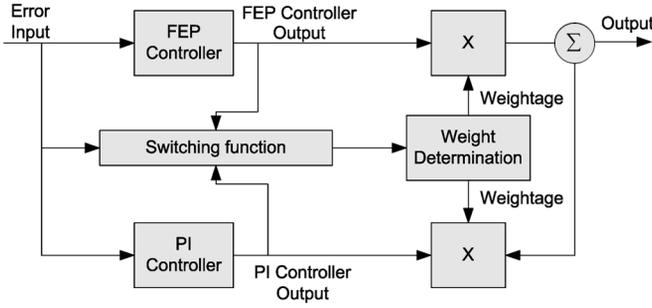
Fig. 1. Schematic diagram of the HPI speed controller with switching function.
