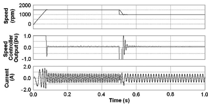
Fig. 7. Reference and actual speed, speed controller output, and line current of the vector-controlled PMSM drive with HPI speed controller with switching function based on the average of output of both the FEP and PI controllers.
