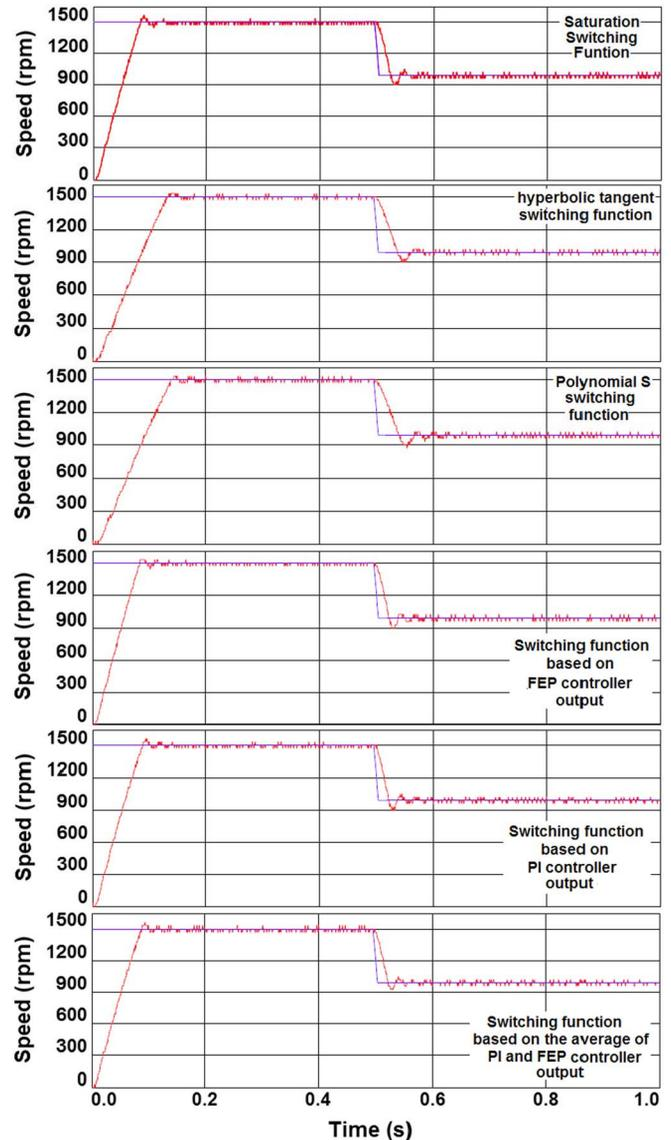
Fig. 8. Experimentally measured speed of the vector-controlled PMSM drive with HPI speed controller with noninherent and inherent switching functions.
