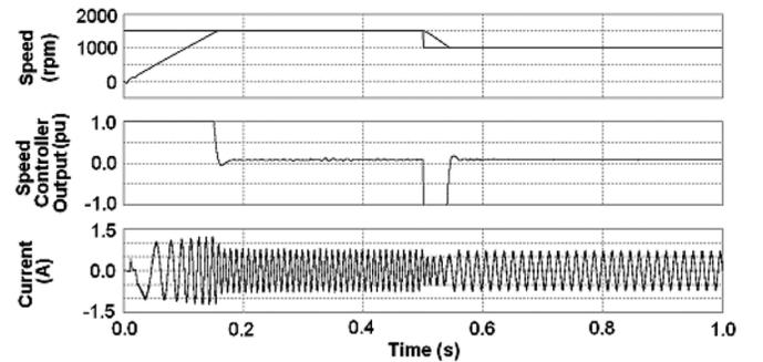
Fig. 4. Reference and actual speed, speed controller output, and line current of the vector-controlled PMSM drive with HPI speed controller based on polynomial S switching function.
