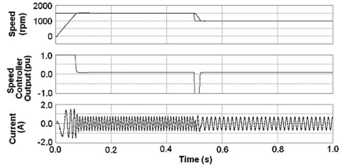
Fig. 3. Reference and actual speed, speed controller output, and line current of the vector-controlled PMSM drive with HPI speed controller based on hyperbolic tangent switching function.
