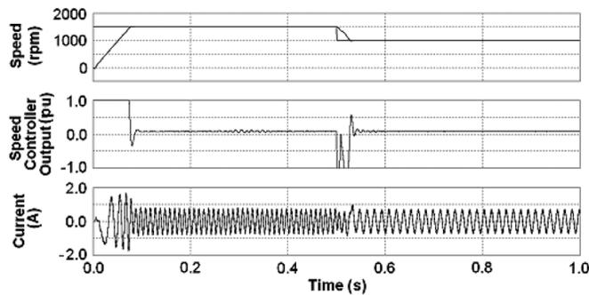
Fig. 6. Reference and actual speed, speed controller output and line current of the vector-controlled PMSM drive with HPI speed controller with switching function based on the output of PI controller only.
