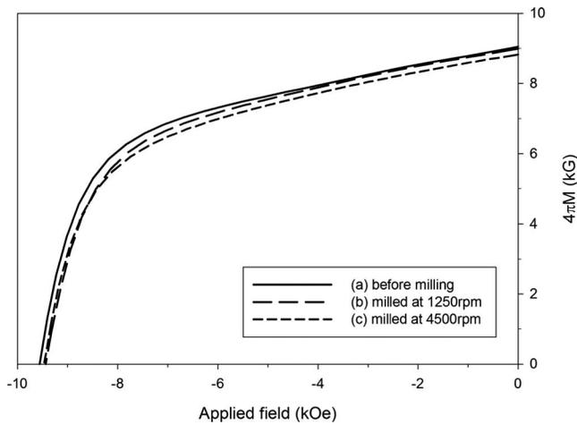
FIG. 4. VSM demagnetization curves of magnet powder (a) before jet milling, (b) jet milled at 1250 rpm, and (c) jet milled at 4500 rpm.
