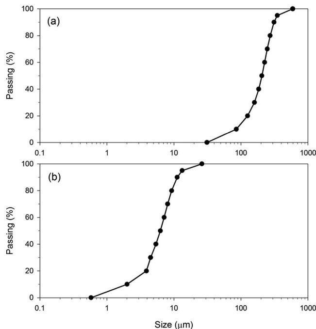
FIG. 3. PSD data of magnet powder (a) before jet milling and (b) after jet milled at 4500 rpm.
