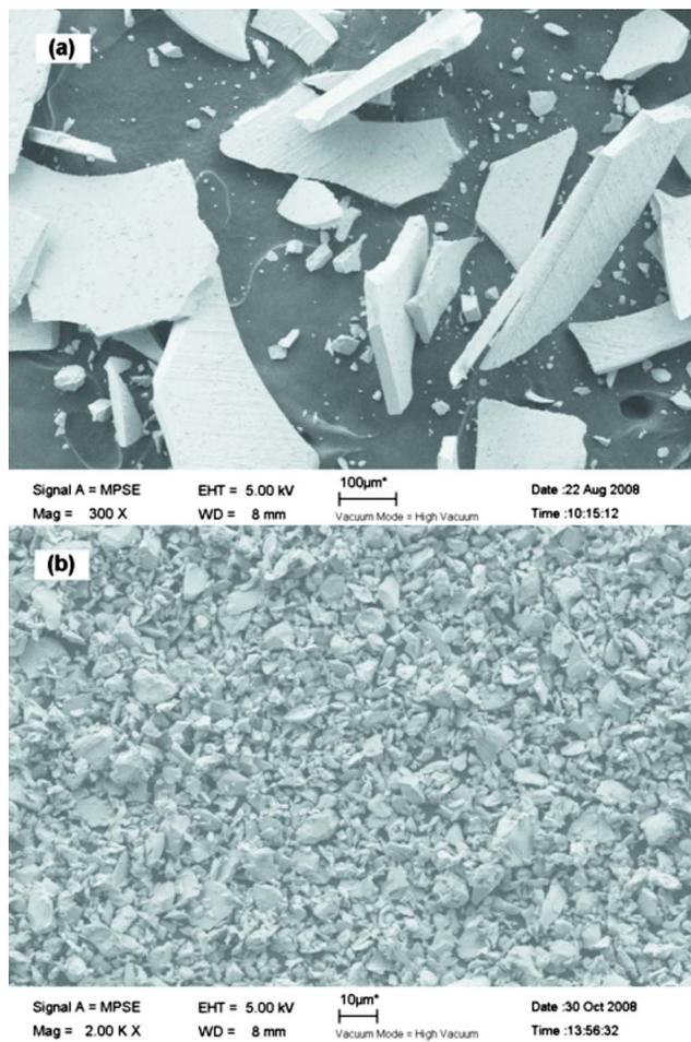
FIG. 2. (Color online) SEM of magnet powder (a) before jet milling and (b) after jet milled at 4500 rpm.
