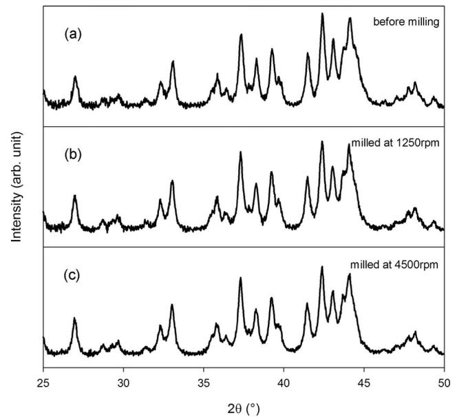
FIG. 5. XRD pattern of magnet powder (a) before jet milling, (b) jet milled at 1250 rpm, and (c) jet milled at 4500 rpm.
