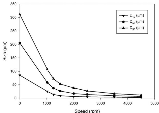
FIG. 1. Powder particle size of jet milled magnet powder as a function of milling speed.
